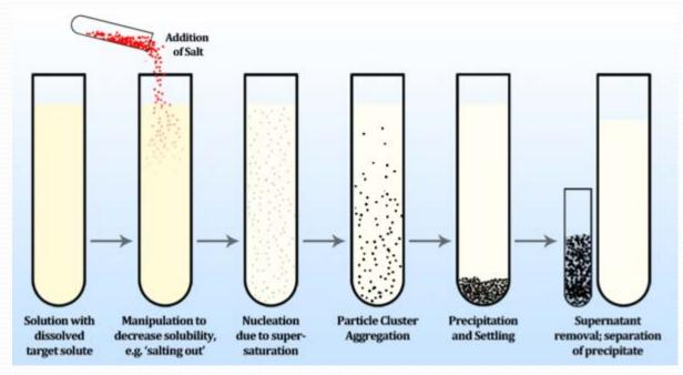
The rate of precipitation of proteins by salt precipitation depends on a number of factors such as hydrophilic properties of the protein, its molecular weight, electric charge; thus the salt precipitation of various proteins occurs in various salt concentrations.
