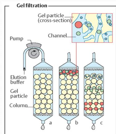
• The speed of micromolecules migration through the column is less than of macromolecules – it allows to purify proteins of micromolecular compounds.
